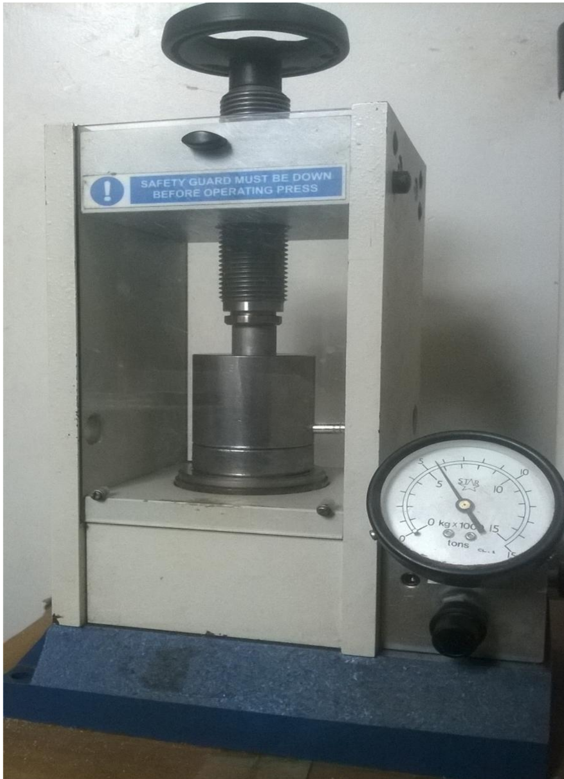
Figure 3.3: Hydraulic press and die assembly used for pelletized solid samples (Source: Self)
